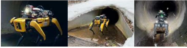
Fig. 3: Active illumination and exposure control on Boston Dynamics Spot and Unitree Go2 robots, inspecting Culvert 110 under Erie Canal.
